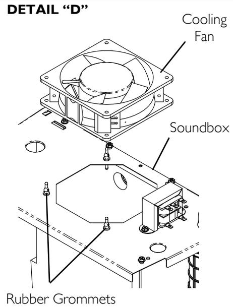
*NOTE: Cooling fan removed from rubber grommets to show proper installation of grommets in soundbox.*
