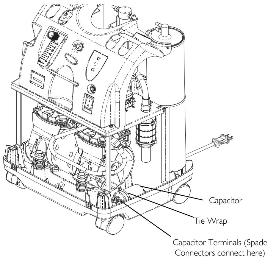
**FIGURE 7.2** Replacing Capacitor
