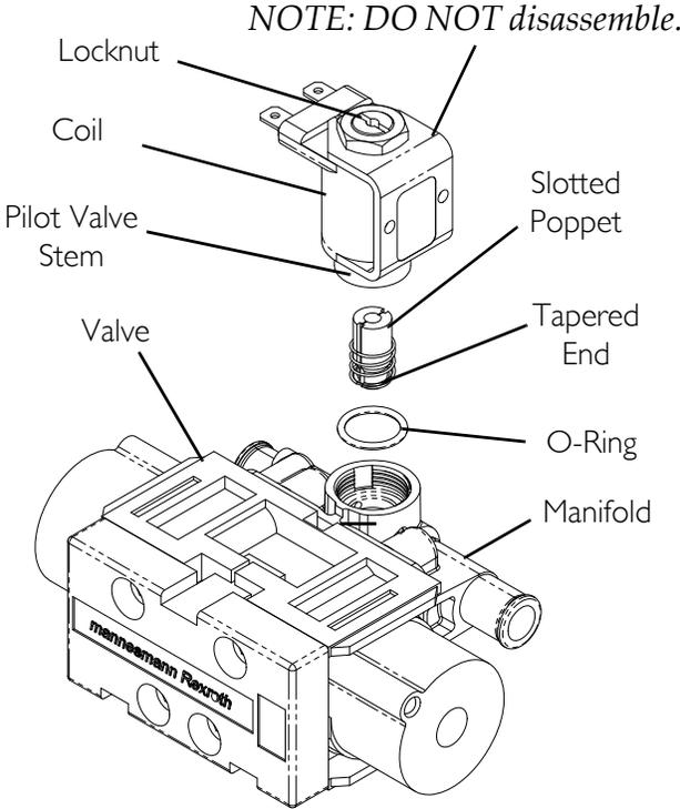
**FIGURE 20.2** Replacing Pilot Valve Poppets and O-Rings
