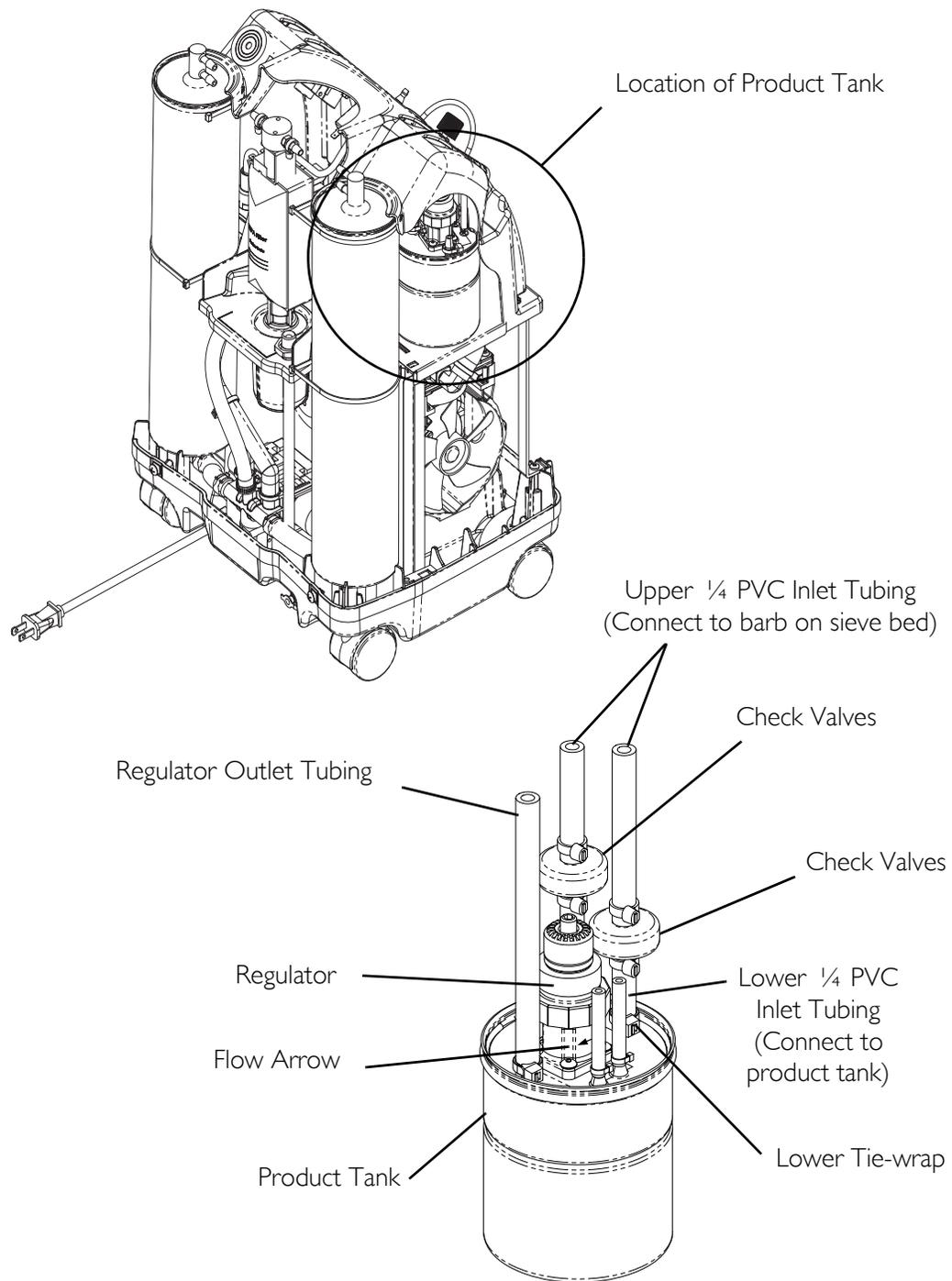
**FIGURE 10.1** Replacing Check Valves
