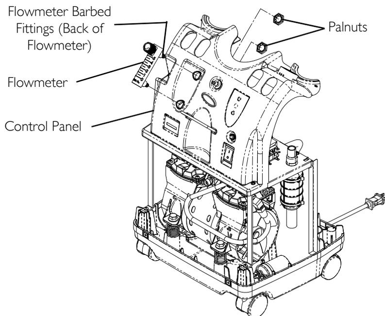
**FIGURE 18.1** Replacing Flowmeter
