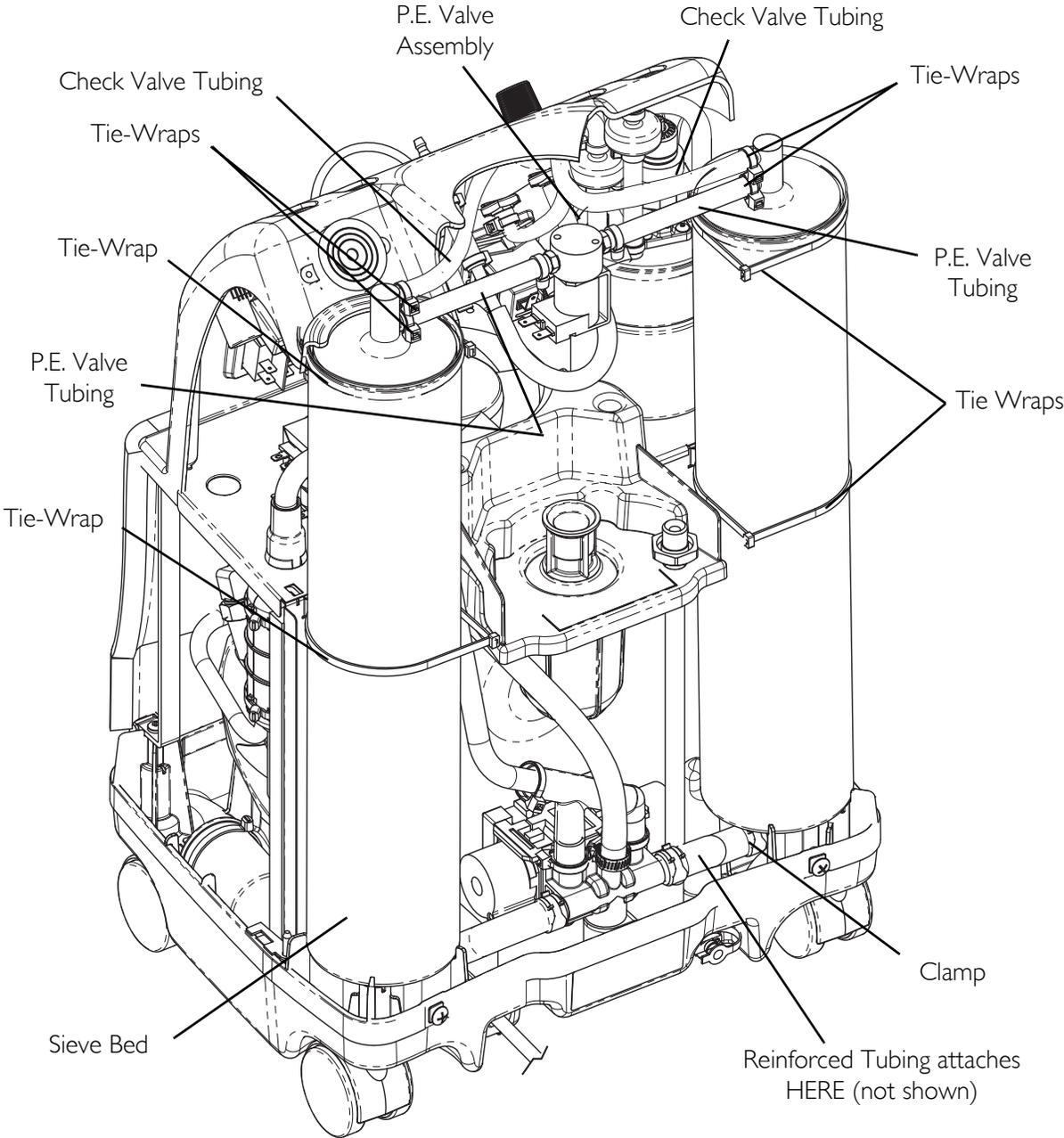
NOTE: Compressor Inlet HEPA Filter removed from illustration for clarity.
