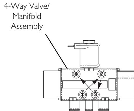
*NOTE: The Numbers above indicate the MOUNTING SCREW TORQUE SEQUENCE: pre-torque to 10 + 2 inch-lbs., then torque to 22 + 2 inch-lbs.*
