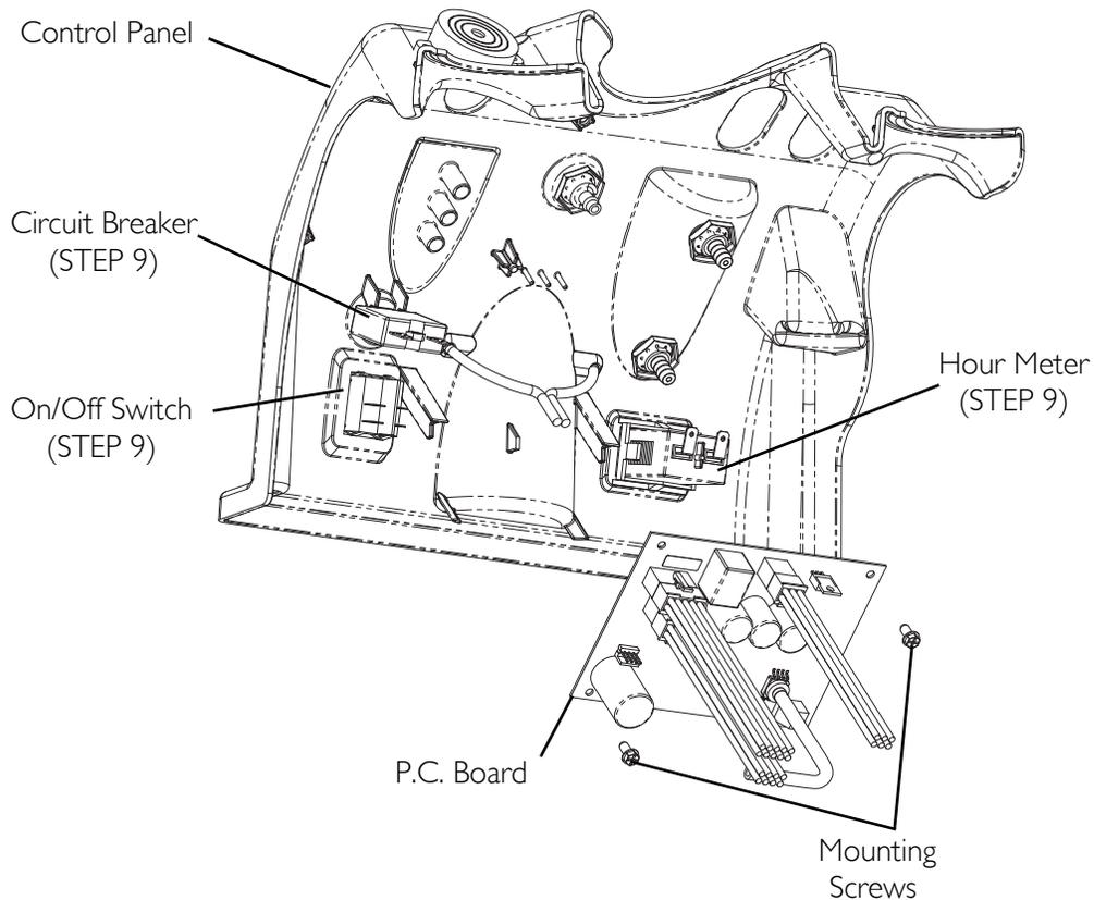
**FIGURE 13.1** Removing Control Panel
