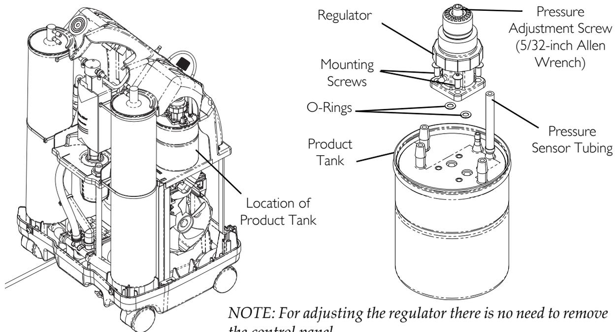
*NOTE: For adjusting the regulator there is no need to remove the control panel.*
