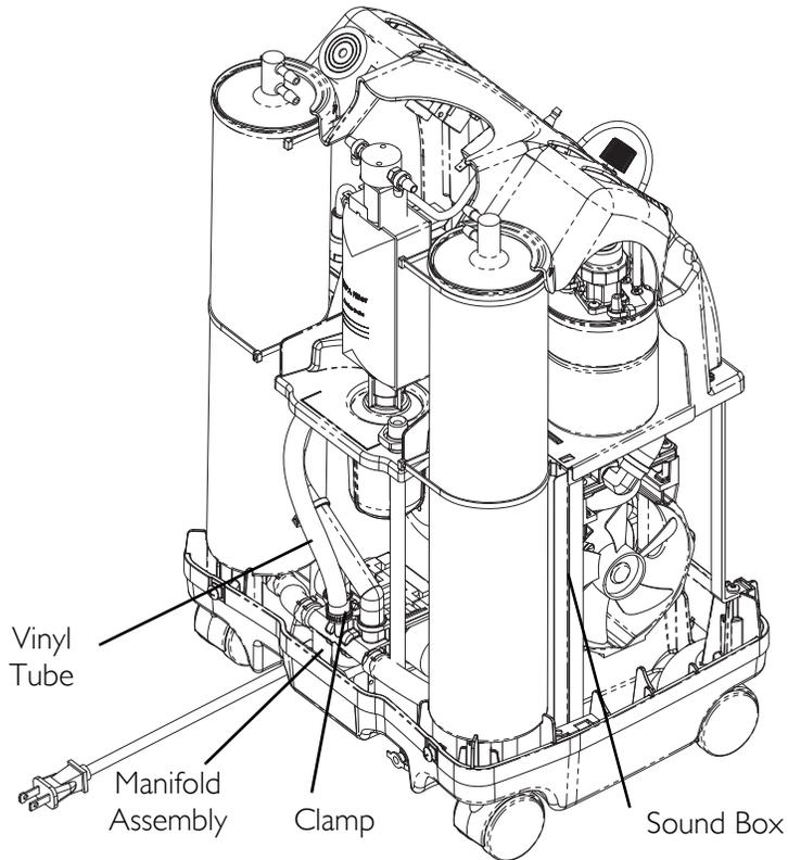
**FIGURE 12.1** Replacing Heat Exchanger Assembly
