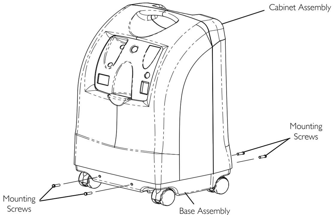
**FIGURE 5.1** Removing Cabinet
