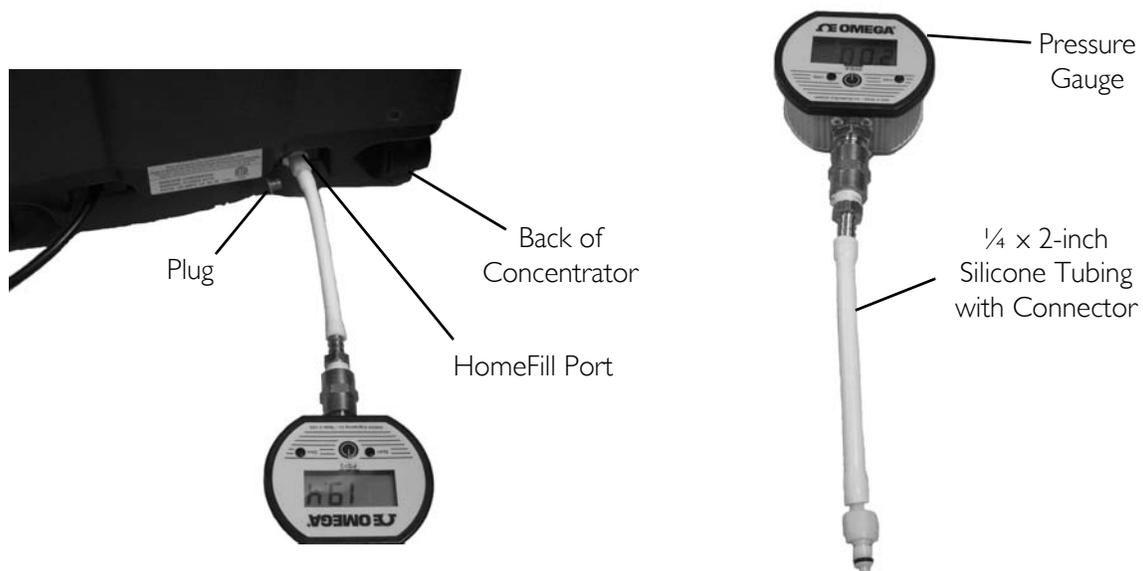
**FIGURE 25.2** Pressure Testing
