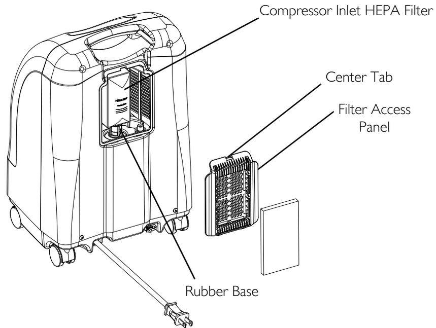
**FIGURE 6.3** Replacing the Compressor Inlet HEPA Filter
